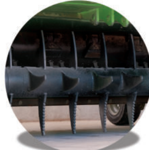
-A rotor with a working width of 200cm. It features 42 conveying blades and 24 shredder blades-
